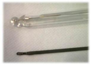
Figure 2: Comparison of a traditional pH glass electrode (above) and an ISFET pH probe with the ISFET sensor on the probe tip (below). Image: Shauna Scanlon.
