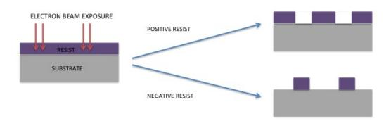
Figure 1: Schematic illustration of development of positive and negative resists after electron beam exposure. Image: Anushka Gangnaik
