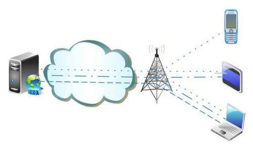
Figure 1: A single SVC stream being transmitted from a celluar tower to three devices each with different capabilities. Image: Jason Quinlan.
